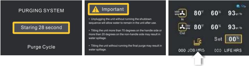
“Pump working countdown”: indicates: No matter in which working state and interface, as long as the pump works, this interface appears and counts down to 28 seconds. However, the interface only displays the previous working status and interface after 3 seconds. For example, after 3 seconds, there is a drainage icon on the main interface and it will flash until the drainage is finished.
