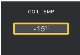
“Coil Temp 000°C ”: Used to display the current temperature of the coil.When it is below zero, the “-” symbol is displayed in front. “.” is not required on zero.
