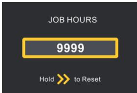
“Indicates”:Do I need to clear out this time?”, press “>”if you need to clear. When the operation is completed, the working time of the main interface and the working time of this interface will be reset and started to be instant again. After accumulation (9999), clean up and round.
