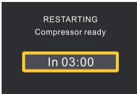
**"Compressor ready IN 03:00"** indicates : That the interface will be displayed when the compression is in a protected state. (including power-on and shutdown, the humidity rises immediately after the arrival of L0 HI, and the shutdown resumes immediately after the emergence of L0 HI).Displays the countdown in seconds.If the above situation does not occur within 3 minutes, it is not shown.
