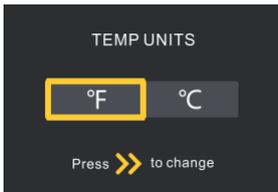
**"Temp Units °F/°C":** Used for temperature scaleswitching.Press the ">" button to switch °F/°C, after switch symbol of corresponding parts is also changing.
