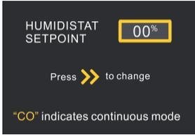
**"Humidistat Setpoint 00%":**Used for setting dehumidification mode humidity.Press ">" to set the humidity. The adjustment range of humidity setting is between 25 and 80%. Each key rises or falls 5%, which can be recycled.
