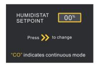
"Humidistat Setpoint 00%":Used for setting dehumidification mode humidity.Press ">" to set the humidity. The adjustment range of humidity setting is between 25 and 80%.
