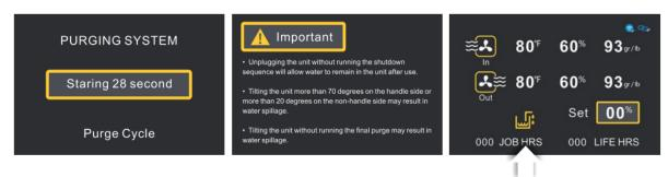
**Pump working countdown:** indicates: No matter in which working state and interface, as long as the pump works, this interface appears and counts down to 28 seconds. However, the interface only displays the previous working status and interface after 3 seconds. For example, after 3 seconds, there is a drainage icon on the main interface and it will flash until the drainage is finished.
