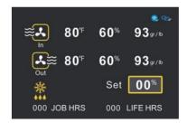
is in the frosting state. At this point, the frosting interface displays 3 seconds, and returns to the submenu program in the background countdown. When the user returns to the main interface without any operation, the frosting state is displayed in the main interface in the way of icon flicker.
