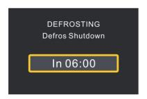
When the machine is running normally, <sup>a</sup>Defrost SHUTDOWN IN 06:00" will occurs in the interface after defrosting. Ifs defrost countdown use seconds as units. This screen displays only 3 seconds. Displays the previous interface and status after restoration. If it is the home screen, the frost icon will flash.
