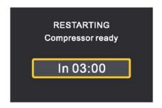
Compressor ready IN 03:00 indicates: That the interface will be displayed when the compression is in a protected state, (including power-on and shutdown, the humidity rises immediately after the arrival of L0 HI, and the shutdown resumes immediately after the emergence of L0 HI). Displays the countdown in seconds. If the above situation does not occur within 3 minutes, it is not shown.
